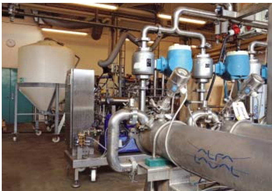
Tests with the new cell removal system using a high-speed separator and cross-flow membranes have been conducted at Alfa Laval's research centre in Naskov, Denmark
