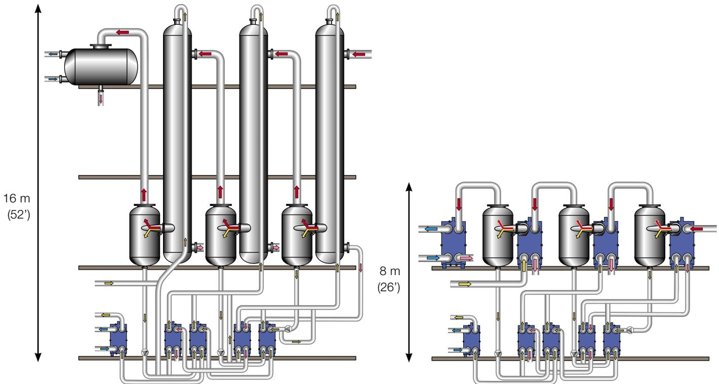
Comparison between shell-and-tube and AlfaVap for a three-effect system that evaporates NaOH from 32 to 50%. The savings in installation costs and space are clearly apparent from the layouts shown above.
