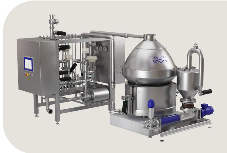
Alfa Laval's eDrive (direct drive) system ensures mechanical simplicity with fewer rotating parts, which prolongs service interval, improves energy efficiency and robustness.
