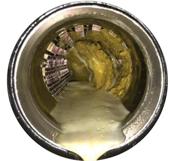
Blockage of heat exchanger downstream of the tank
