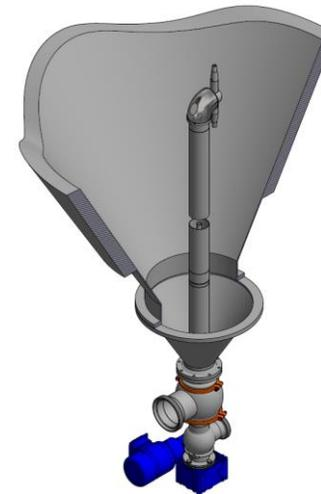
Cutaway of IMXD installation on tank dosing point
